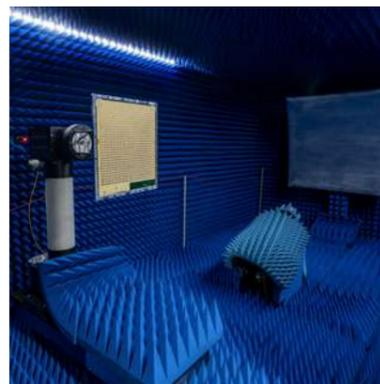
The Advanced RF Testing Chamber with Phased Array Antenna Module.
